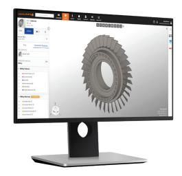
Paperless Parts also analyzes 3D CAD models based on various manufacturing processes like CNC machining or sheet metal fabrication to identify potential issues like tight corners, deep holes that require special tooling, and bend reliefs. The manufacturability detection thresholds can be customized to your shop's capabilities to provide critical insight into how you want to price a specific part.
